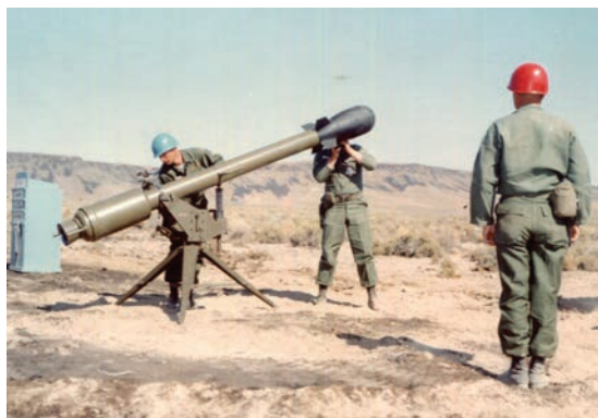
Among the smallest of the weapons in the Army's nuclear arsenal was the M28/M29 Davy Crockett, a recoilless rifle system operated by a three-man crew. It entered into service in the early 1960s (Photo provided by Los Alamos National Laboratory Historical Department).
